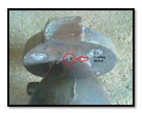
Figure 1. Defective Globe Valve
