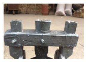
Figure 15. Modified gating system part
