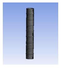
Fig. 3 Meshing of CHS sections
