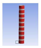
Fig.2. CFRP wrapped specimen
