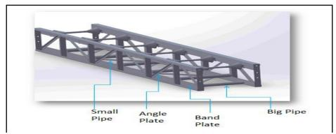
Figure 9: Modeling of modified all section
