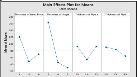
Figure 5 Main effect plot for mean data - shear stress
