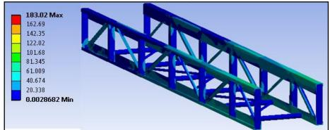
Figure 10: Shear stress in modified section
