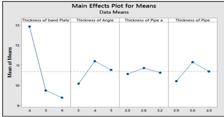
Figure 7 Main effect plot for mean data - deflection
