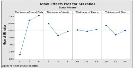
Figure 8 Main effect plot for S/N ratio data – deflection
