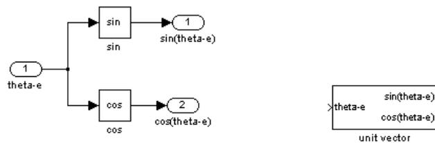
Figure 9. Unit vector simulink block.
