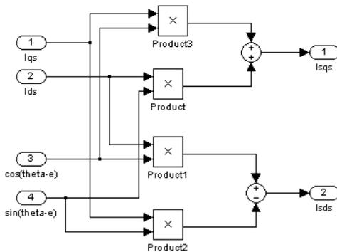
Figure 16. syn-abc-1 conversion simulink block.
