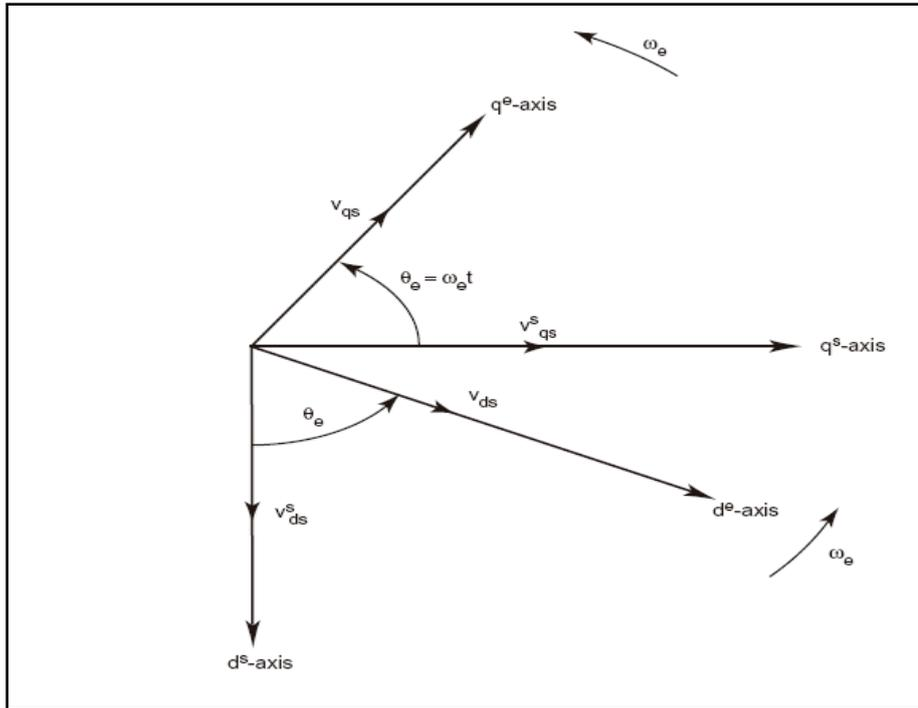
Figure 2. Stationary frame to synchronously rotating frame transformation.
