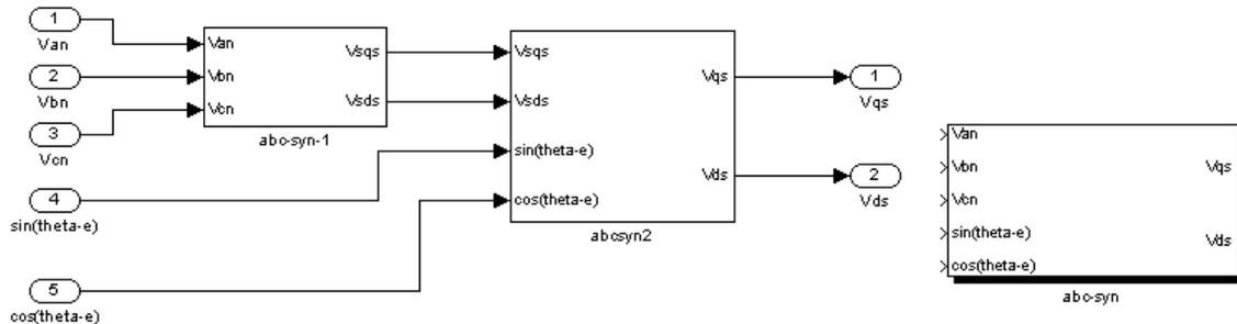
Figure 10. abc-syn conversion simulink block.
