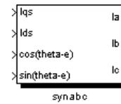
Figure 14. Syn-abc conversion simulink block
