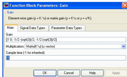
Figure 17. syn-abc-2 conversion simulink block.
