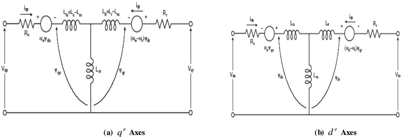
Figure 3. Dynamic  $d^e - q^e$  equivalent circuit of machine.
