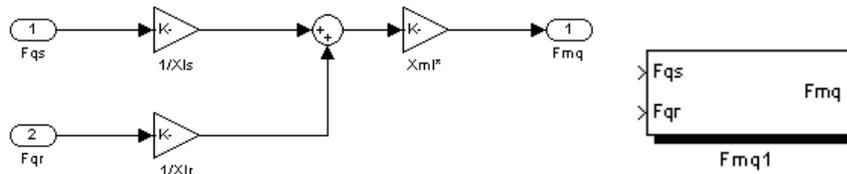
Figure 29. Fmq matlab simulink block.
