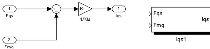
Figure 33. Iqs matlab simulink block.
