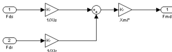
Figure 27. Fmd matlab simulink block.
