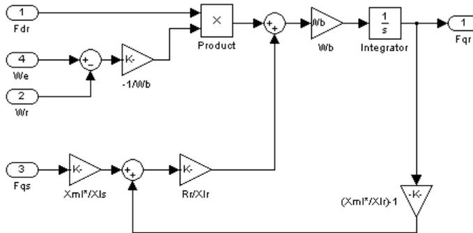
Figure 23. Fqr matlab simulink block.
