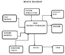
block diagram of gas leakage detection and control
