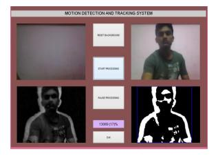
Fig. 4 Human is detected (i.e Blob is detected)
