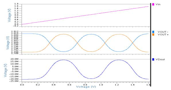
Figure 5 DC Simulation Results of Folding Amplifier using 0.18um technology (Vin 1.6V)
