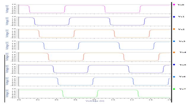
Figure 11 Cyclic thermometer code of Fine converter
