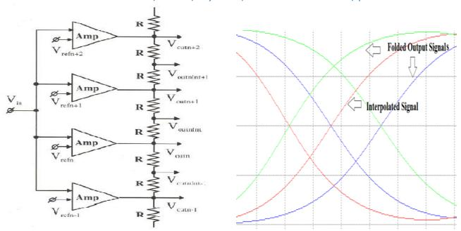
Figure 7(a) Implemented resistive interpolation technique
