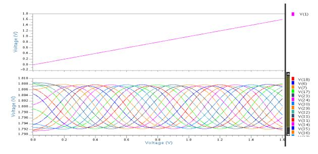
Figure 8 Zero crossing points using folding & interpolation techniques
