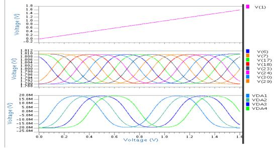
Figure 6 Generated Sixteen Zero Crossing points using four parallel folding amplifiers
