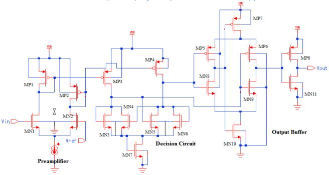
Figure 9 High Performance Voltage Comparator [3][17]
