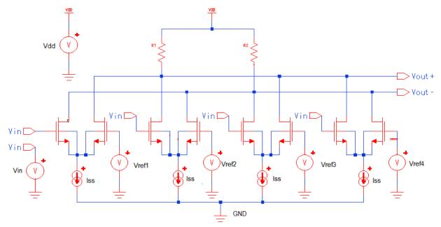
Figure 4 Folding amplifier with folding factor=4 [6]
