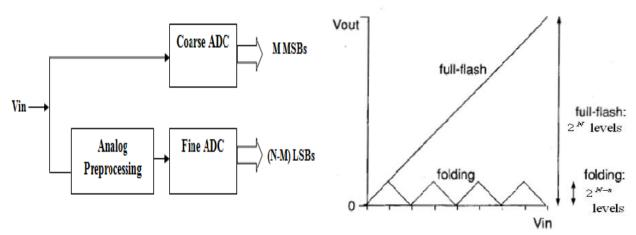
Figure 1 Block Diagram of folding ADC
