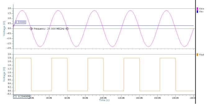
Figure 10 Transient analysis of comparator
