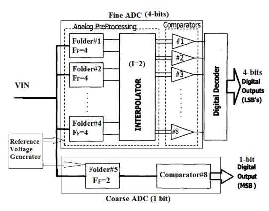
Figure 3 Architecture of 5-bit folding & interpolating ADC
