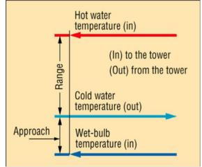
Figure 2 Cooling Tower: Range and Approach
