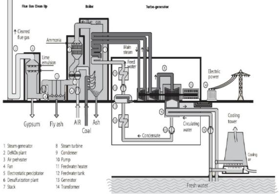
Figure 1. Diagram of a Typical Coal-fired Thermal Power Station
