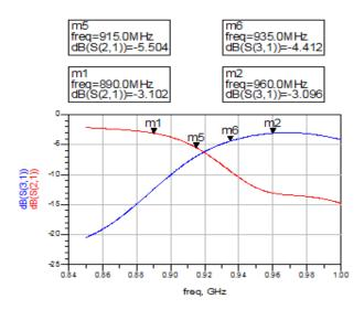
Figure8. Transmission loss of the duplexer
