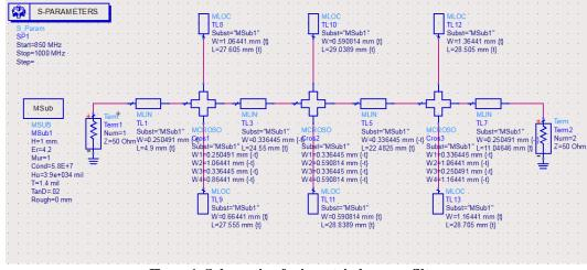
Figure 1. Schematic of microstrip lowpass filter
