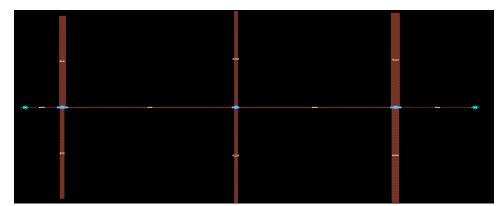
Figure 2. Layout of microstriplowpass filter
