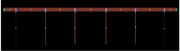
Figure 4. Layout of microstrip highpass filter
