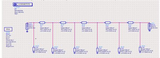
Figure3. Schematic of microstrip highpass filter
