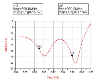
Figure 9. Return loss of the duplexer
