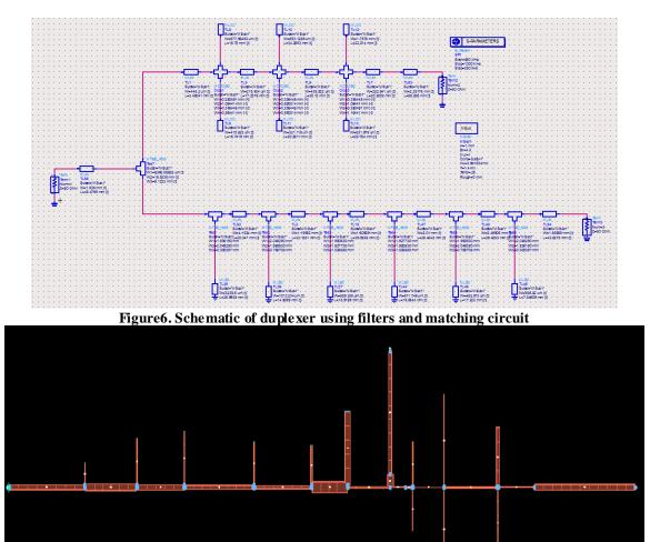
Figure 7. Layout of duplexer using filters and matching circuit IV. SIMULATION RESULTS
