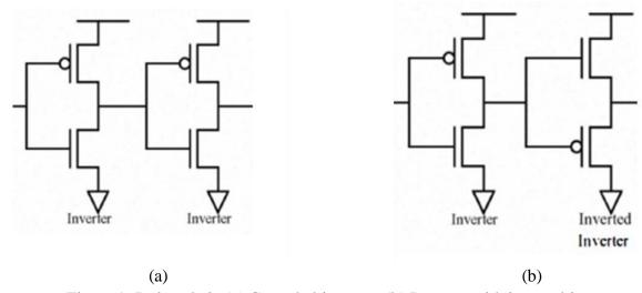
Figure 1: Delay chain (a) Cascaded inverter, (b) Inverter with inverted inverter
