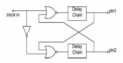
Figure 2: Block diagram of non-overlapping clock generator
