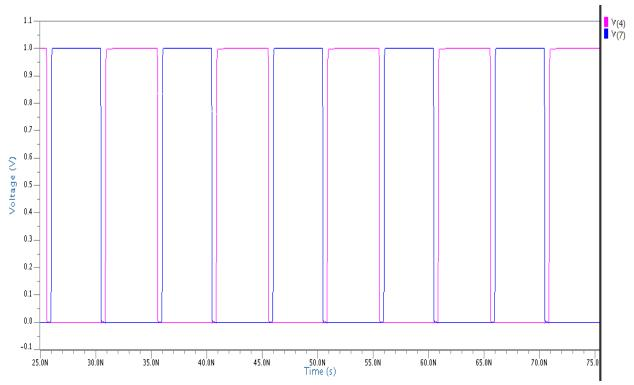
Figure 5: Non overlapping clock signals using inverted inverter
