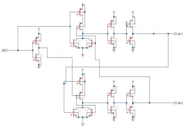
Figure 4: Non overlapping clock generator using inverted inverter
