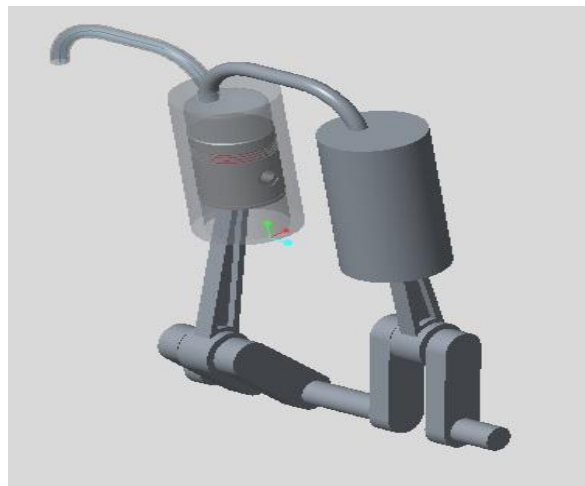
Figure 2: Assembly model of six stroke engine
