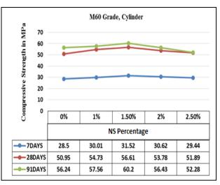
Figure 3: Compressive Strength of Cylinder M50 Grade Figure 4: Compressive Strength of Cylinder M60 Grade
