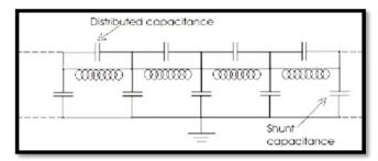
Figure 3. Distributed RLC network of transformer
