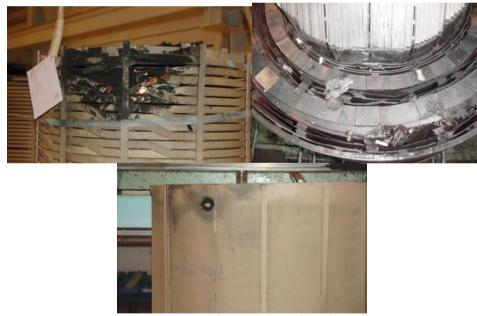
Figure 5. Problem in core and winding
