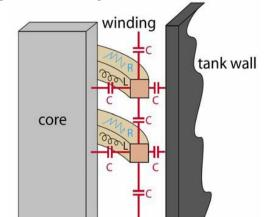
Figure 2. The simplified network behavior of a transformer's active part
