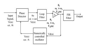
Fig. 1 Block diagram of FM receiver
