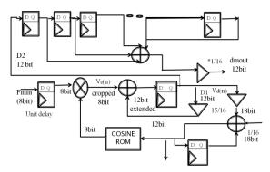
Fig. 7 Complete block diagram of all digital FM receivers
