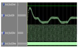
Fig.11 Simulation waveform for NCO
