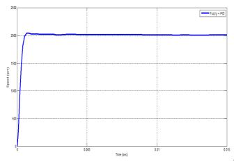
Fig. 8 : response of the Fuzzy + PID Logic for speed set at 2000 rpm
