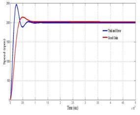
Fig. 3: Responses of PID Controller
