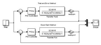
Fig. 2: Simulink model for the closed loop PID controller
