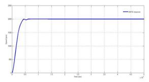
Fig. 5 : response of the Fuzzy Logic Control for speed 2000 rpm
