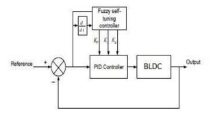
Fig. 6: Block diagram of Fuzzy + PID Controller
