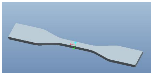
Figure 2 3-D CAD model Specimen for Tensile testing
