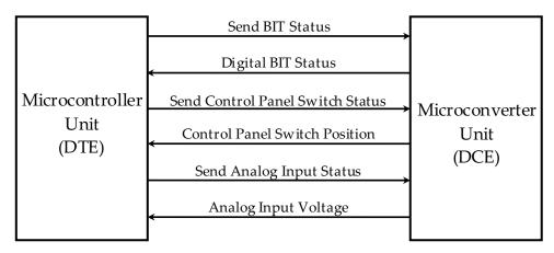
Fig.2 – Serial Communication between DTE and DCE
