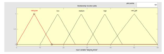
Figure 5. Input membership function of last time vehicles
