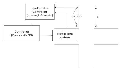
Figure 3. General structure of a traffic lights control system
