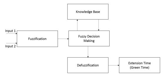
Figure. Building block diagram of a Fuzzy Logic Controller
