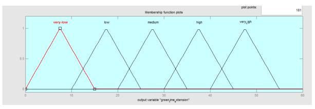
Figure 6. Membership function of output (green time extension)
