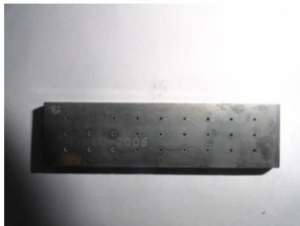
Fig 1: Final micro hole Drilled Components
