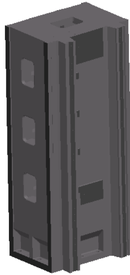
Figure-3. Structure Modeling Of VTL Column
