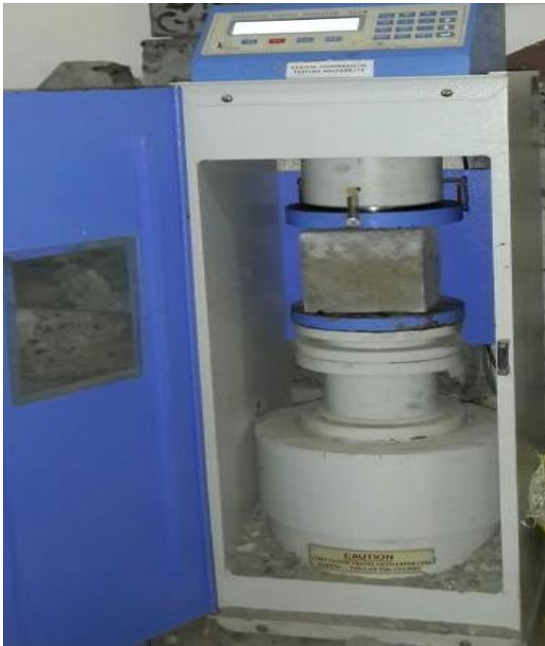
Figure 3:- Compressive Test Apparatus Figure 4:- Effect of Used Waste Plastic on Compressive Strength
