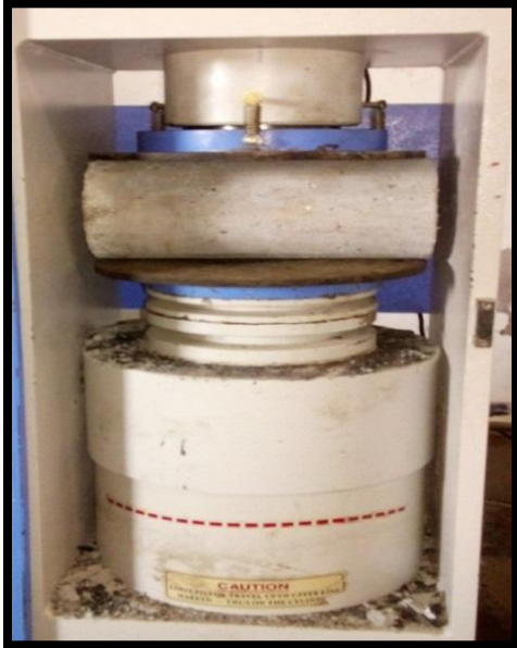
Figure 5:- Split Tensile Strength of Concrete
