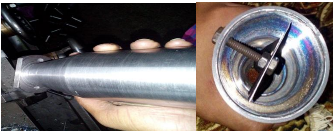
Figure 7:- Newly designed internally threaded inlet manifold with swirling device at centre
