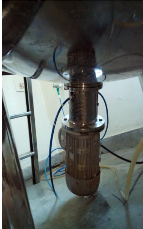
Figure 10. Agitator having one impeller blade mounted at bottom of tank at 45 0 angle
