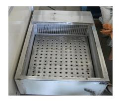
B) **NORMAL** (**COOLING**) **WATER CURING:** After the cube specimens were prepared, they left to stand undisturbed in their moulds in place free from vibration at a temperature of 27 ±2<sup>0</sup>C for 1 day from the time of addition of water to the ingredients. Then remove from the mould and specimens are lowered into the curing tank and it is remain totally immersed for a period of 7 & 28 days. Then results were observed.
