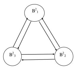
Fig.3. Digraph representing sub-factors affecting cutter runout: 1 uncut chip thickness, 2 shear angle 3 friction angle
