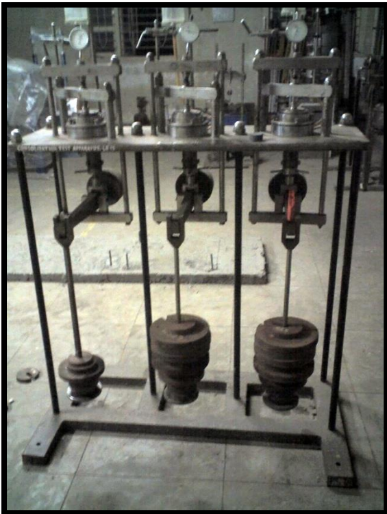
Figure 1. Consolidation test set up
