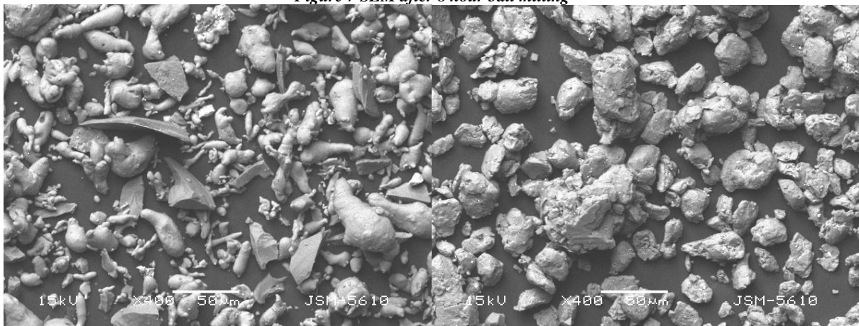
Fig 8 SEM data of hand mixing Al-SiC powder
