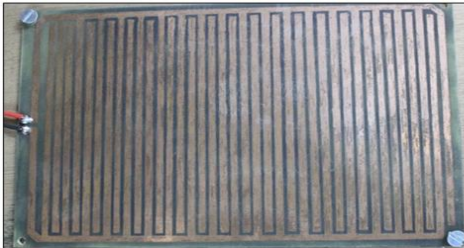
Fig. 1. Moisture Detection Sensor etched on a copper PCB
