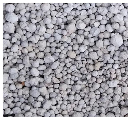
Plate 2. Pelletized Silica fume aggregate
