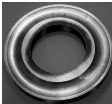
Fig. 6: Ovality defect in bearing ring
