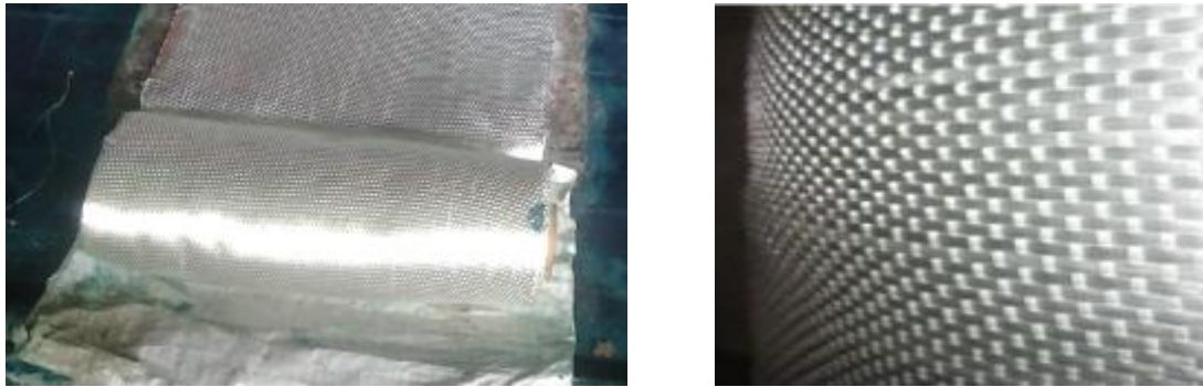
Fig. 2. GFRP Sheet (a) Sheet roll and (b) Unidirectional GFRP sheet
