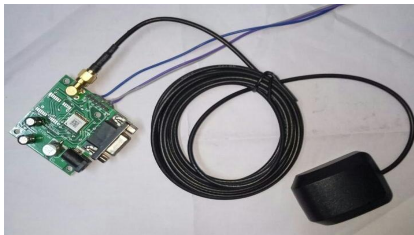
Figure 4: GPS Modem with external antenna
