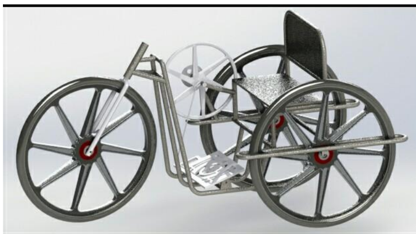
Figure 2. Tricycle with sewing machine mechanism
