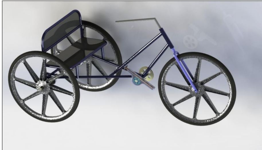
Figure 7. Design Model of handicapped tri-cycle
