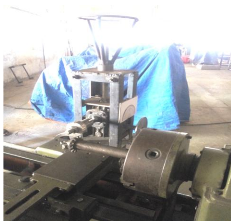
Figure 1. Gear cutting attachment for lathe.
